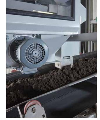
The inline test device QualiMaster ATI removes samples immediately downstream of the mixer from above the conveyor. As an option, a sample crusher can be incorporated in the basic version ATI Eco.
