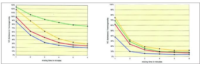
Blue = EIRICH mixer horizontal pan Red = Turbo mixer / Turbine type mixer Blue = EIRICH mixer inclined pan
